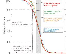
Comparison virtual-impactor with main PM<sub>2.5</sub> separator
